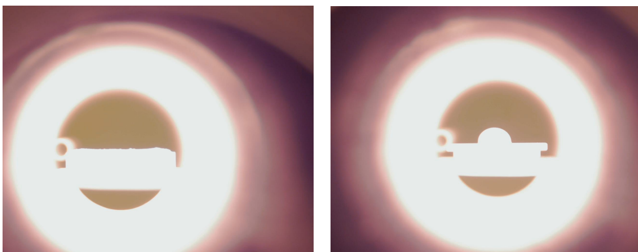
Figure 2. Photographs of reactivity tests between refractory crucibles and bulk highlands melt after 1 hour (alumina; left) and 25 hours (boron nitride; right) at 1600 °C.
